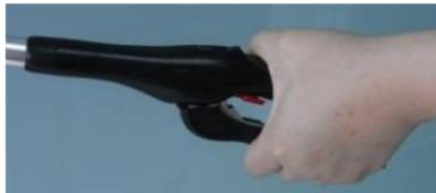
14. After firing, release the firing handle, and allow it to return to its original position. After the handle is released, return the safety to the locked position.
