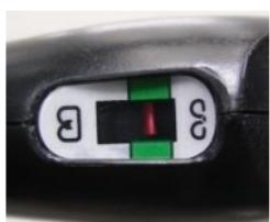
12.Prefire checklist : The Red line is in the middle of the green bar. The anvil is securely attached.To fire the instrument, pull the red safety back toward the wing-nut until it seats into the body of the instrument.
