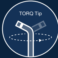
TORQ Tip Shape for Circumferential Sweep
